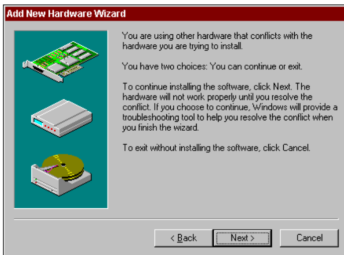
Figure 2-5. AT-GPIB/TNT Resources Not Assigned Successfully
