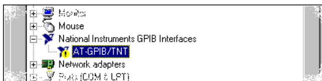
Figure 2-16. GPIB Interface That Is Not Working Properly
