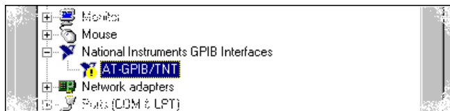
Figure C-1. GPIB Interface That Is Not Working Properly
